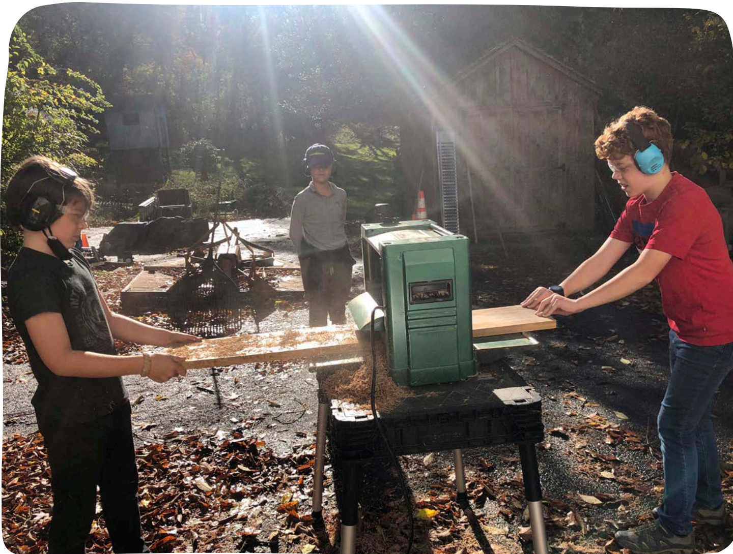
Carter watches while Ollie and Max plane down a piece of maple that will be used to make cutting boards. The Planer smooths the surface of the board.
